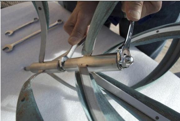
Now upright, it's time to change the bearing at the top of the sculpture, which you can access by removing the top rounded or "acorn" nut. As before, brace the sculpture and keep it steady with your 9/16" wrench on the top middle nut while you unscrew the top acorn nut.
