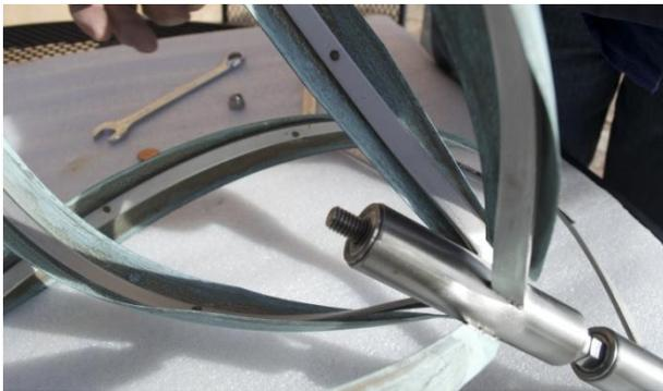
The top of the thread rod will be exposed, along with the lip of the bearing, shown to left.
