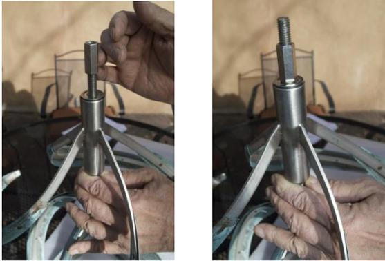
Replace your long connector nut by twisting it onto the thread rod with your fingers at first, then with the 9/16" wrench, until the connector nut is all the way down the rod and touching the bearing. Now you can flip over your sculpture.
