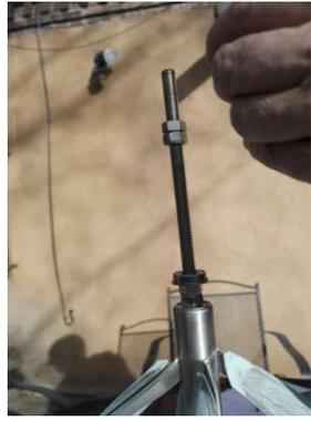
Now your second bearing is visible and will easily slide off the thread rod, allowing you to slip on a new bearing. After the new bearing is in place, replace the two nuts almost but not quite halfway down the length of your thread rod, leaving them loose until you're sure they're resting at the right spot on the pole.
