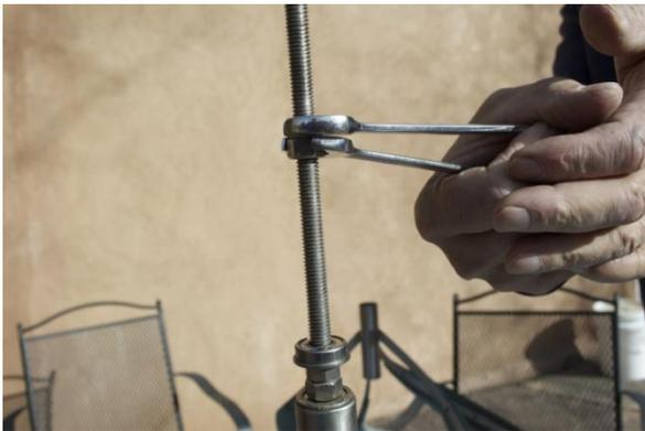
Use two 9/16" wrenches to untwist the two nuts. To do this, you will apply pressure to each nut from opposing directions. Remove these two nuts and set them aside.
