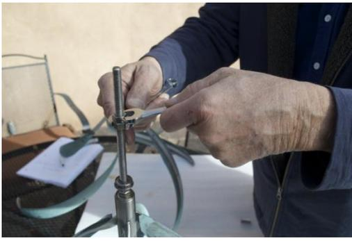
Once you're sure the distance between the bearing and sculpture opening is correct, it's time to tighten the two nuts back into place with your two 9/16" wrenches. Slide the sculpture back onto the thread rod, over the two nuts; slide the new bearing over this.
