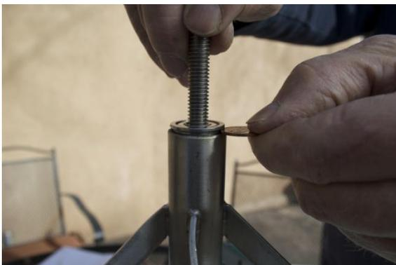
You can tell whether the distance is correct once you slip the bearing over the thread rod, down to the base of this layer of sculpture. If correct, a penny will fit between the lip of the bearing and the stainless opening of the sculpture.
