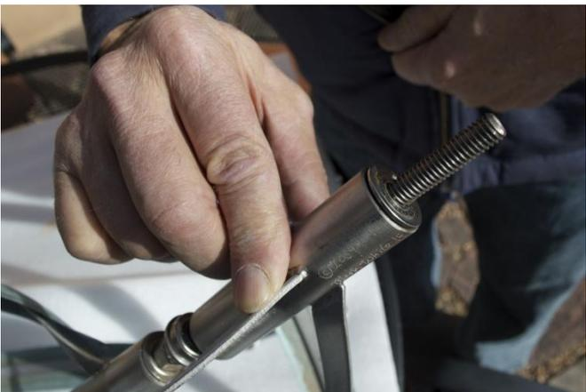
Once this connector nut has been removed, your thread rod will be exposed as shown in the picture at left, with the top of the bearing visible.
