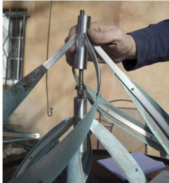
Slip over the bottom half of your sculpture until it rests on the lip of the bearing and the two lower nuts below the bearing.
