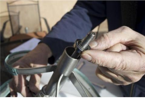
Slide the bearing up and off of the thread rod.
